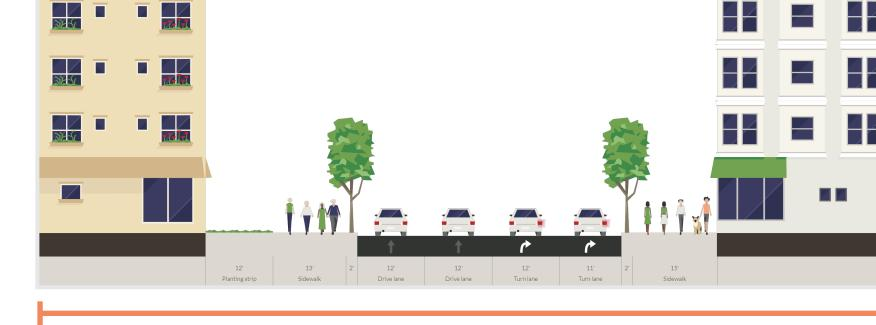
Option 1: Buffered Bike Lane & Road Diet Road Diet: Removing one travel lane per direction.
